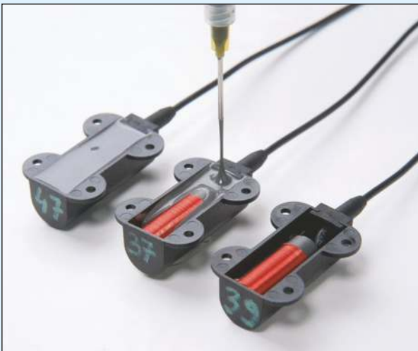
Potting of electronic components
